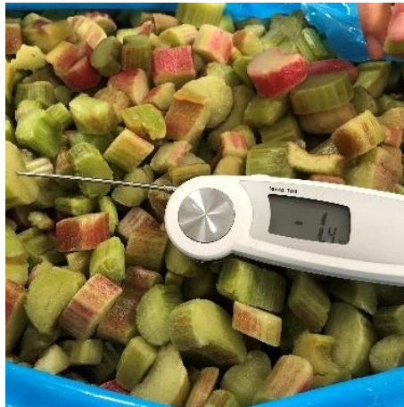
Rhubarb 100 kg bags (10 x 10 kg) 1000 kg/h from -18 °C to -3 °C/-1 °C
