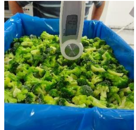
Broccolis 200 kg bags (10 x 20 kg) 1700 kg/h from - 18 °C to - 3 °C/- 1 °C
