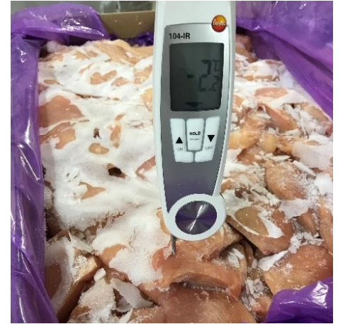
Chicken breasts 150 kg (10 x 15kg) 1500 kg/h from -18°C to -4°C/-2°C Block size: 600 x 400 x 260 mm
