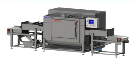
The very low floor space, the length under microwaves (residence time) and the crossed coupling of microwaves above and below the blocks, are a few examples of the solutions used to conciliate capacity, flexibility, efficiency and homogeneity.
